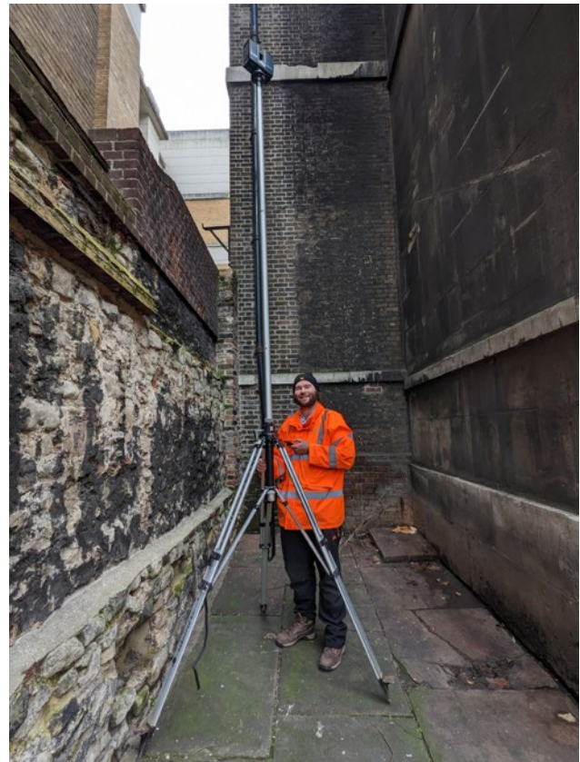
A terrestrial scanner attached to a telescopic mast helps capture every level of St Mary Abchurch including its tower.
