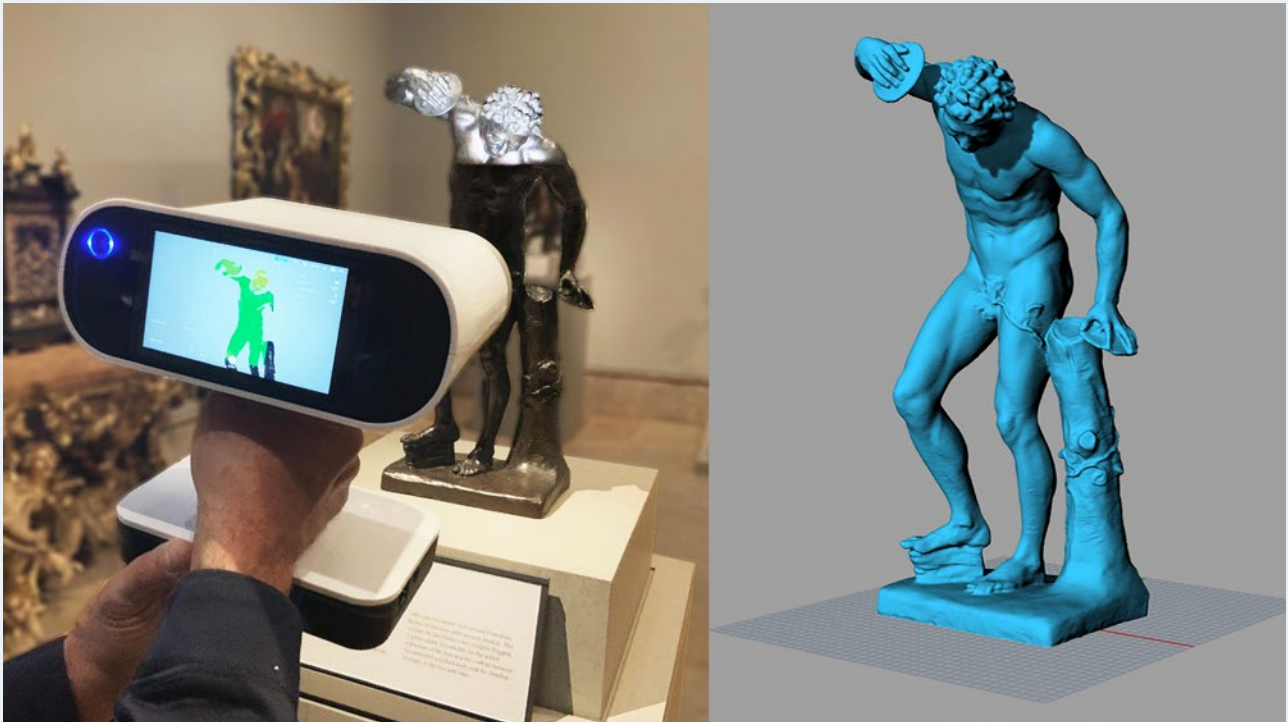
Museum conservation staff use scanning to acquire accurate, non-invasive three-dimensional data about a bronze sculpture (left), and after processing produce a digital 3D model (right).
