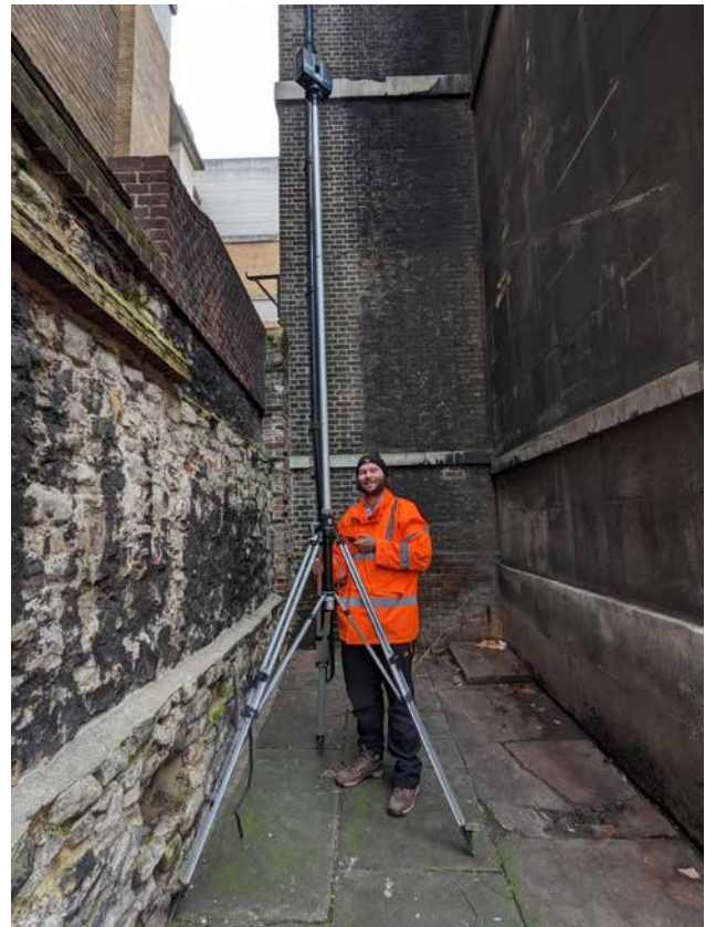
A terrestrial scanner attached to a telescopic mast helps capture every level of St Mary Abchurch including its tower.
